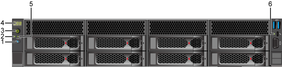
Figure 5-12 Indicators and buttons on the front panel of the 4-GPU server
