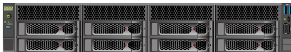
Figure 5-28 8 x 3.5" drive configuration
