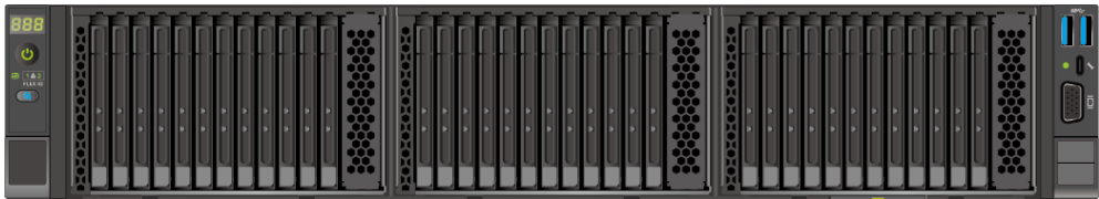
Figure 5-24 36 x E3.S 1 T pass-through configuration
