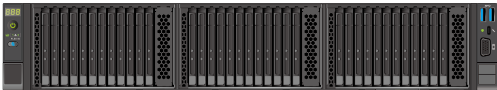
Figure 5-36 36 x E3.S 1 T pass-through configuration
