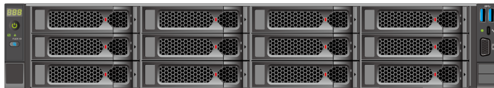
Figure 5-17 12 x 3.5" drive configuration
