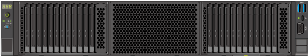
Figure 5-9 24 x E3.S 1 T pass-through configuration
