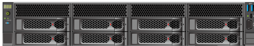
Figure 5-16 8 x 3.5" drive configuration
