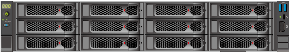
Figure 5-5 12 x 3.5" drive configuration
