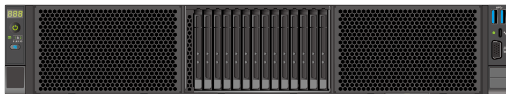
Figure 5-18 14 x E3.S 1 T pass-through configuration
