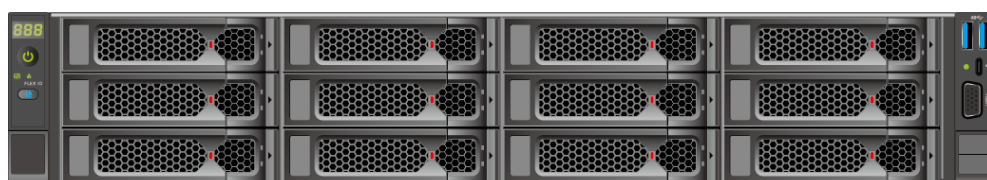
Figure 5-29 12 x 3.5" drive configuration
