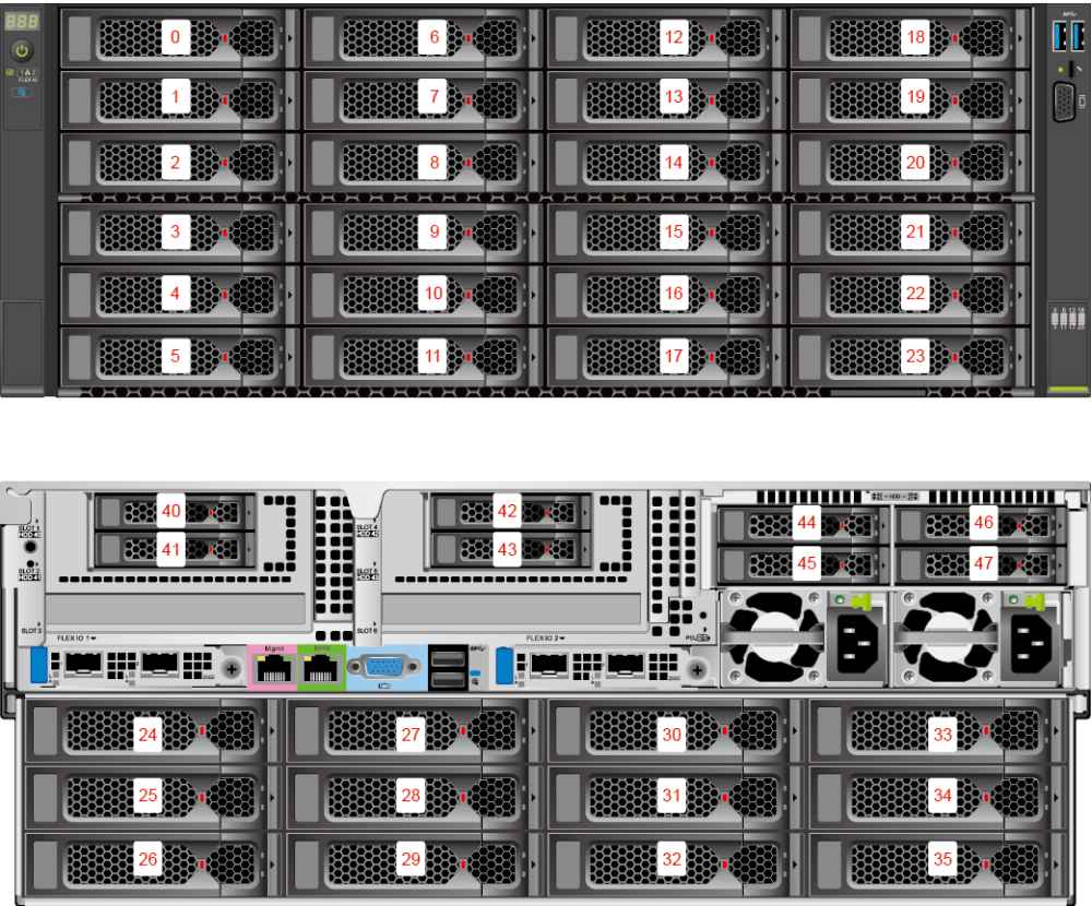
Figure 5-21 Drive numbering (I/O module 1 configured with 2.5" drives + I/O module 2 configured with 2.5" drives + I/O module 3 configured with NVMe drives)
