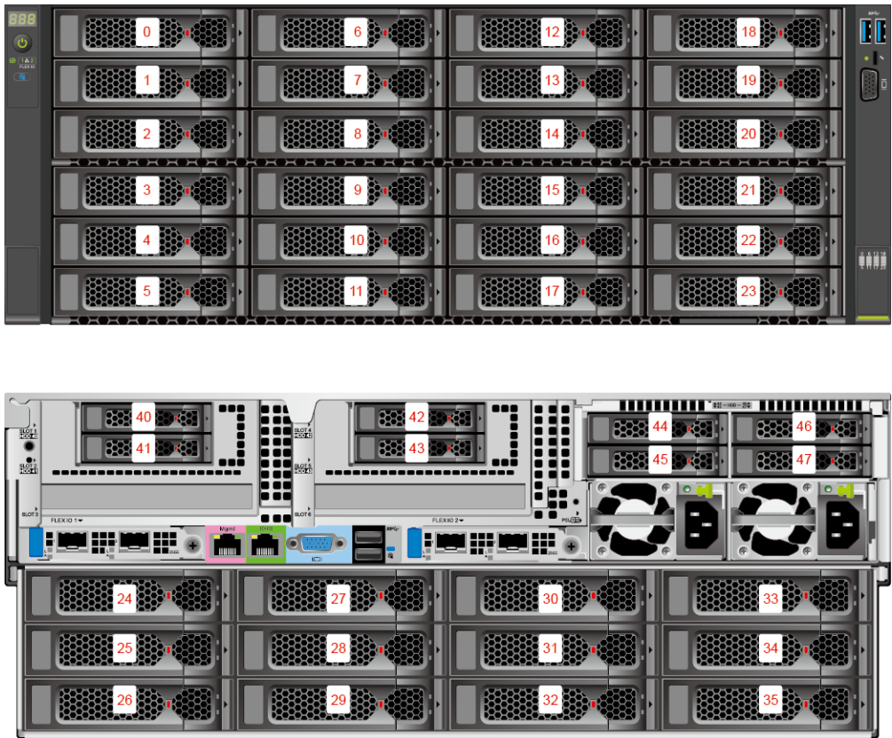
Figure 5-25 Drive numbering (I/O module 1 configured with 2.5" drives + I/O module 2 configured with 2.5" drives + I/O module 3 configured with NVMe drives)
