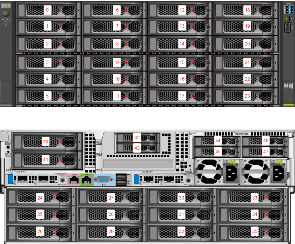
Figure 5-14 Drive numbering (I/O module 1 configured with 3.5" drives + I/O module 2 configured with 2.5" drives + I/O module 3 configured with NVMe drives)
