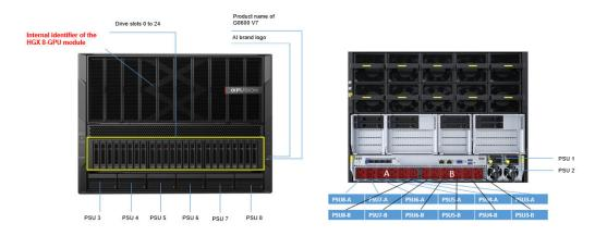
As shown in **Figure 7-1**, the six PSU slots in the front view are for the 54 V dual-input PSUs, which are named PSU 3, PSU 4, PSU 5, PSU 6, PSU 7, and PSU 8 from left to right and are inserted and removed from the front of the server. The two PSU slots on the right in the rear view are for the 12 V single-input PSUs, which are PSU 1 and PSU 2 from left to right and can be removed and inserted from the rear of the server.
