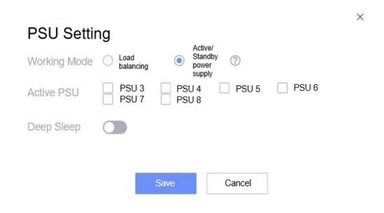
**Load balancing** and **Active/Standby power supply** for PSUs 3 to 8 can be set on the web interface. If **Load balancing** is selected, PSUs 3 to 8 carry the load evenly. To set to active/standby power supply, select **Active/Standby power supply** and select PSUs as the active PSUs to implement different backup modes. The backup modes can be set to N+1, N+N, or N+M.
