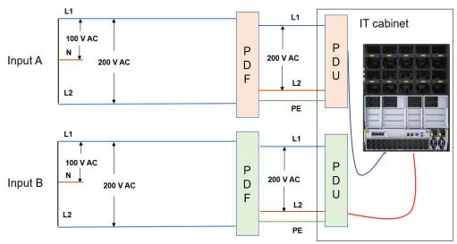
As shown in **Figure 8-2**, dual live wires are used for power supply. Since each input to the power distribution frames (PDFs) has 100 V AC line-to-neutral voltage and 200 V AC line-to-line voltage, the PDFs provide 200 V AC power to the PDUs and then to the PSUs. In this case, the loading capability of the 54 V PSUs is 3000 W and that of the 12 V PSUs is 3000 W. Therefore, the dual-live wires can greatly improve the server configuration.
