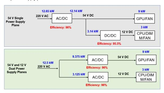
As shown in **Figure 4-1**, the 54 V and 12 V dual power supply planes save 150 W energy compared with the 54 V single power supply plane in the case that the server work load is 12 kW.
