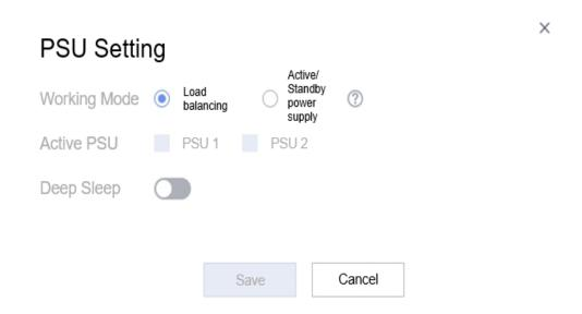
**Load balancing** and **Active/Standby power supply** for PSU 1 and PSU 2 can be set on the web interface. **Load balancing** indicates that PSU 1 and PSU 2 each carry 50% load. To set to the active/standby power supply mode, select **Active/Standby power supply** and select **PSU 1** or **PSU 2** as the active PSU. The active PSU carries 100% load, and the standby PSU does not carry load.
