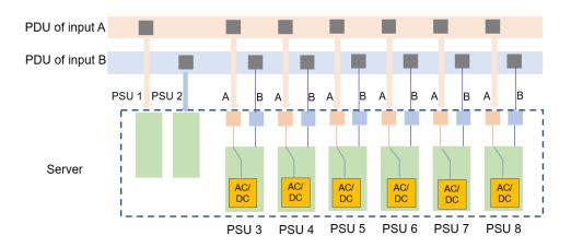
In this mode, the 54 V dual-input PSUs obtain power from PDU A.
