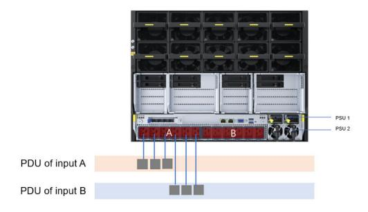
The 54 V dual-input PSUs are also compatible with single input in N+N mode. As shown in **Figure 7-6**, the dual-input PSUs 3 to 8 use only input ports As which connect to the corresponding PDUs of inputs A and B. Input port B of each PSU does not need to be connected.
