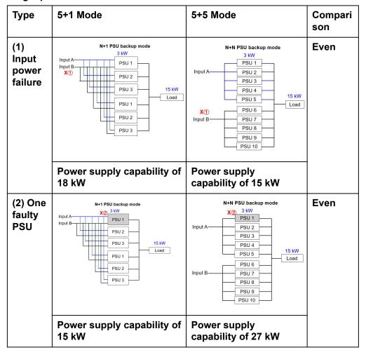
**Summary of reliability upon single-point failure**: The system is designed based on 15 kW. In the N+N and N+1 modes, no matter one input or one PSU
