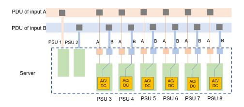
In this mode, the 54 V dual-input PSUs obtain power from PDU B.
