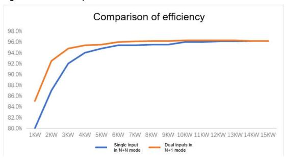
The PSUs have the highest efficiency at 50% load.
