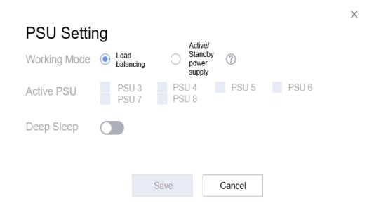
Figure 7-9 Setting the 54 V PSU backup mode 2
