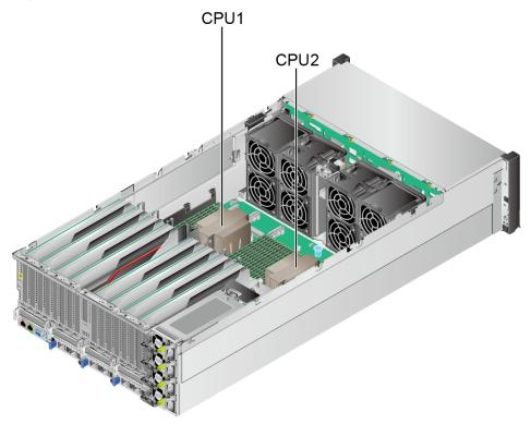
Figure 5-10 Positions of the processors
