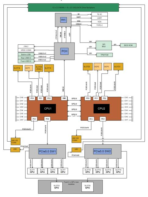
**Figure 4-2** Logical structure 2 (configuration with 20 x 2.5" drives + 10 x dual-width GPUs + 1 x PCle switch board)
