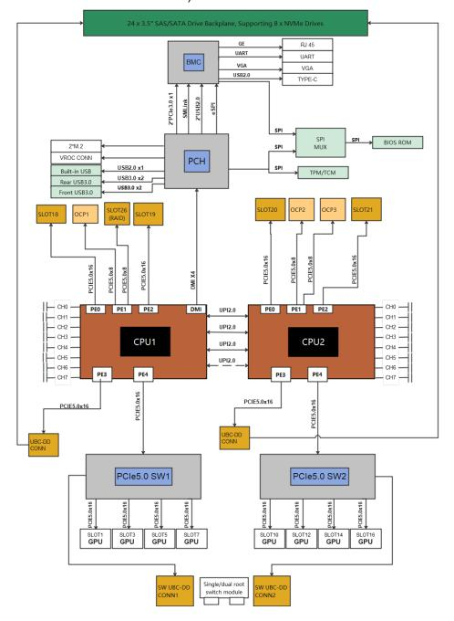
**Figure 4-1** Logical structure 1 (configuration with 24 x 3.5" drives + 8 x dual-width GPUs + 1 x PCle switch board)
