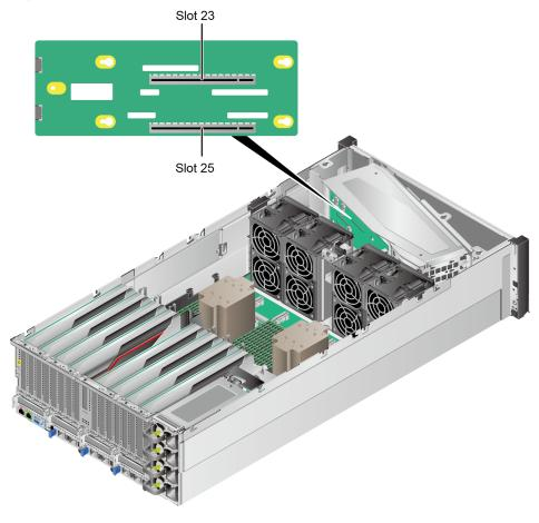
Figure 5-21 Front PCIe slots
