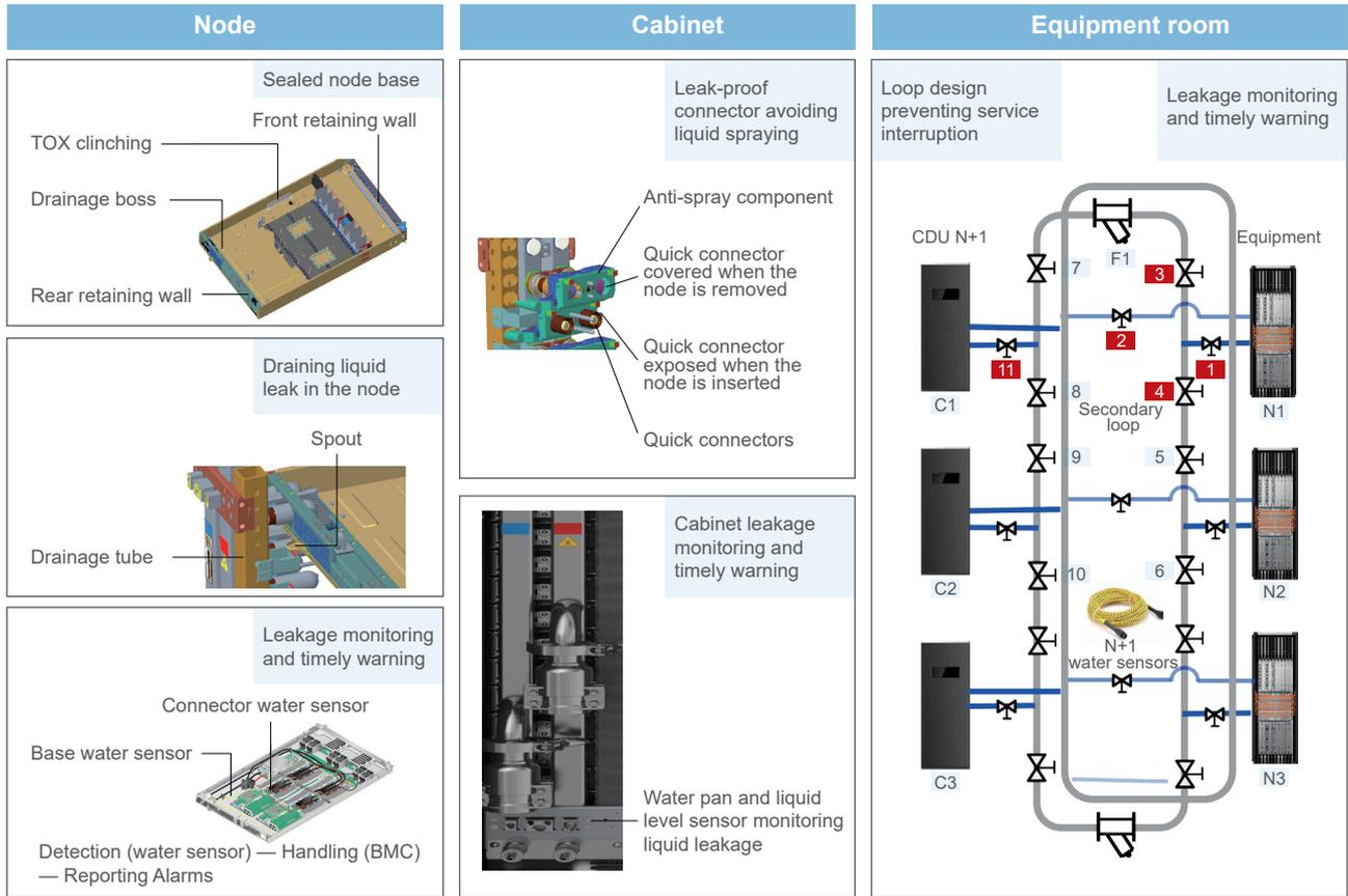
**Figure 3 Main structure of a node, a cabinet, and an equipment room (example)**
