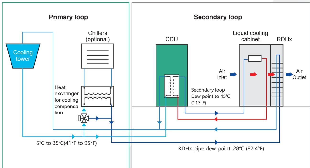
Figure 1 Cooling architecture of a liquid-cooled data center (example)
