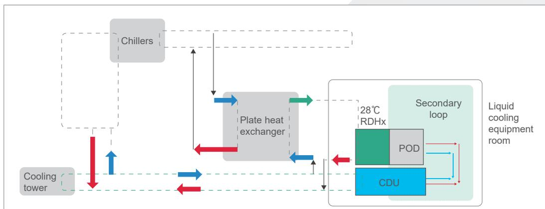
Figure 2 Cold-plate liquid cooling architecture (example)
