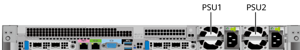
Figure 5-39 Positions of PSUs
