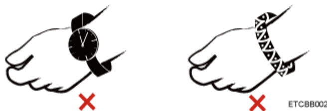
Figure 8-2 Removing conductive objects
