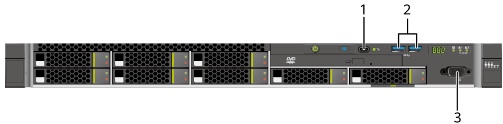
Figure 5-8 Ports on the front panel
