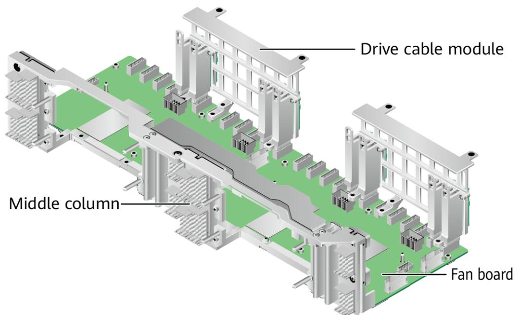
**Figure 5-15** Middle module (24 x 2.5" drive configuration)
