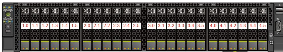
Each server node manages six drives. Drives from left to right are managed by server node 1, server node 2, server node 3, and server node 4 in sequence.
