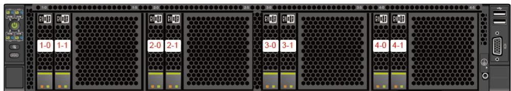
Each server node manages two drives. Drives from left to right are managed by server node 1, server node 2, server node 3, and server node 4 in sequence.
