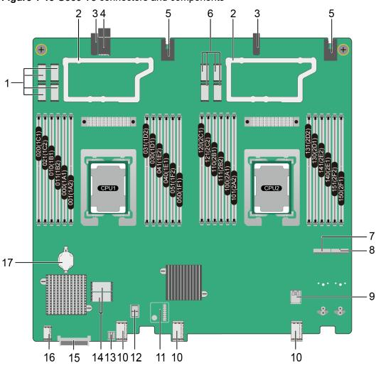
Figure 1-13 G560 V5 connectors and components
