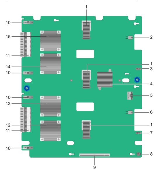
Figure 1-17 Positions of connectors and components on the GS608 PCIe plate
