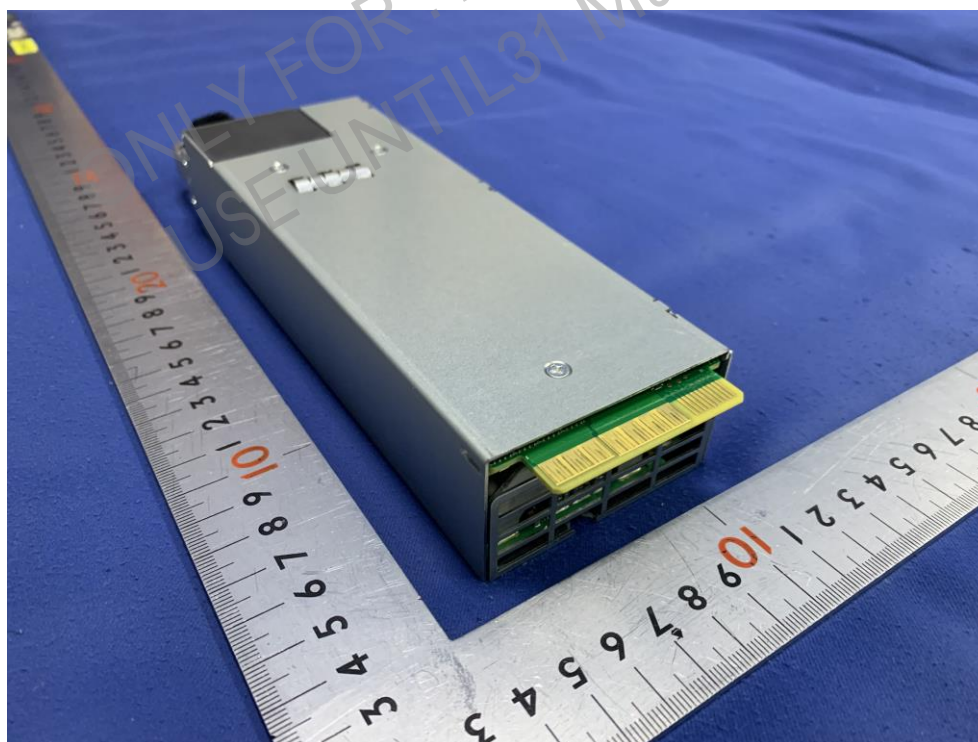
Figure 10– overall view of PSU (PAC2000S12-T1)
