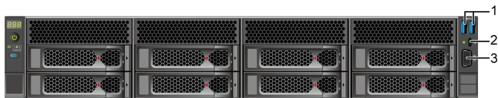
Figure 5-13 8 x 3.5" drive configuration
