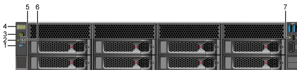
Figure 5-7 8 x 3.5" drive configuration
