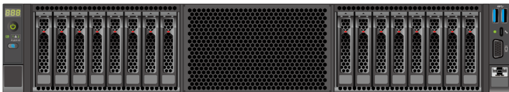
Figure 5-5 16 x 2.5" drive configuration 2
